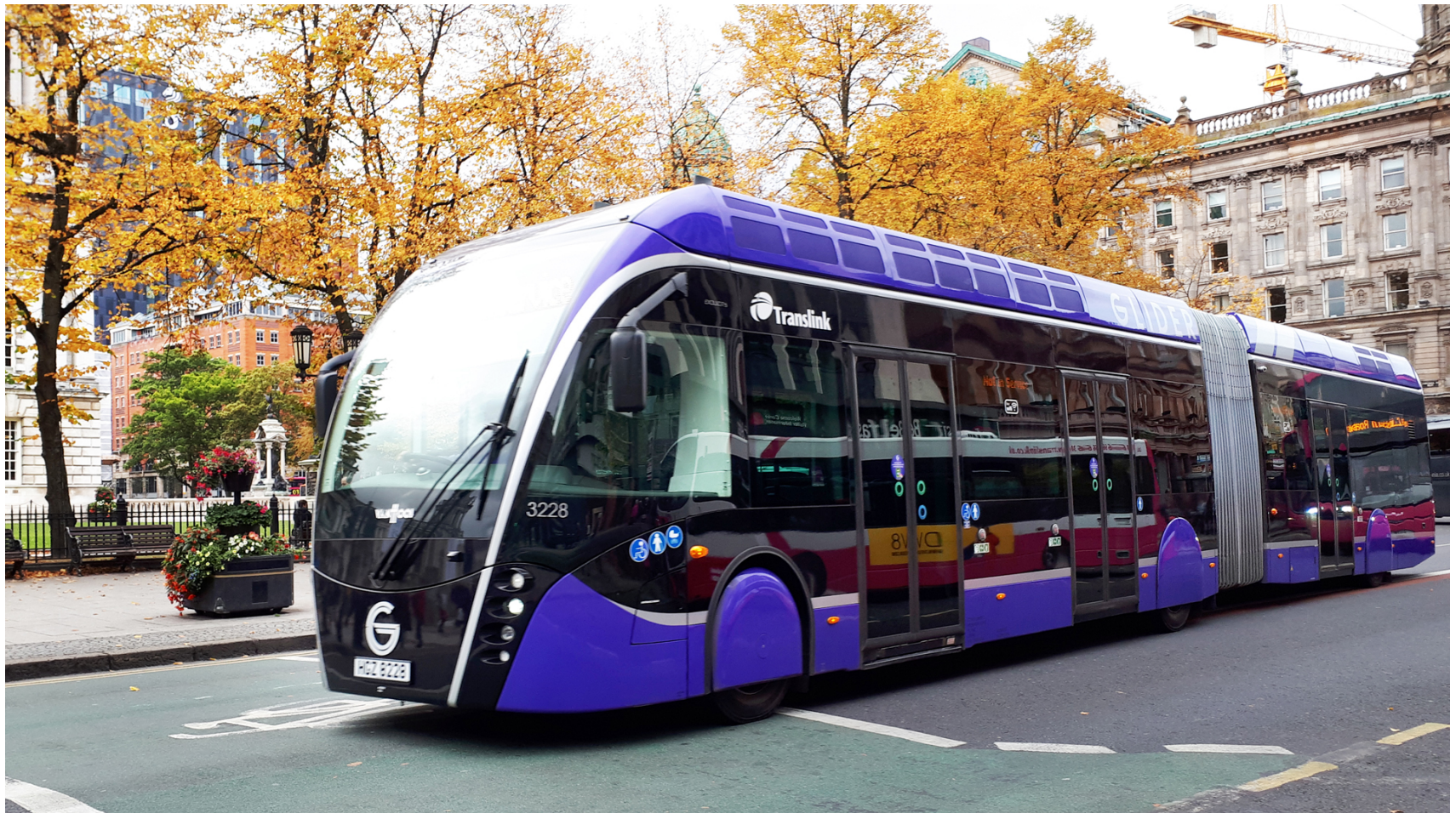
Belfast Glider - Van Hool ExquiCity 18 articulated buses of a light tram design with three doors and approximately 18 metres in length.
